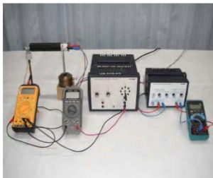
Figure 2. Setting up the experimental verification of Stefan-Boltzmann's law of radiation.
